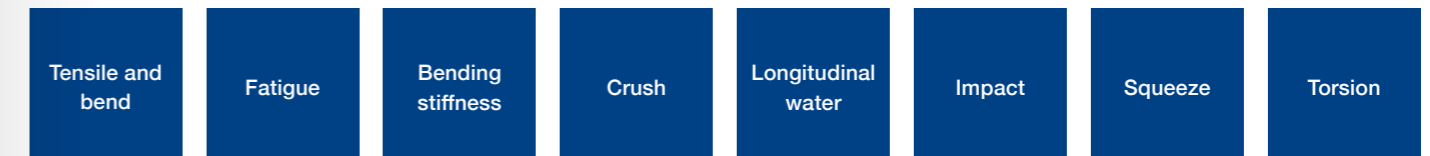
NKT performs several mechanical tests to qualify cable designs, thus reducing project risk during the installation phase.
