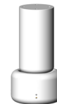
ECDI IEC Extension adapter will extend the insert depth to 757 mm, to meet dimensions according to fluid-type design, Figure 3 in IEC 62271-209.
